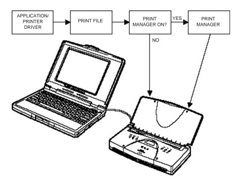
Because most of the time it takes to print is actually the processing time needed for the computer to prepare the print file, background printing does not usually give you any real advantage.
